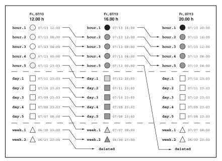
The snapshots marked with black symbols are newly created at the respective point in time (e.g. 16.00 h). The snapshots with icons filled with dark-gray are files from the previous backup run (e.g. for the 16.00 h backup this is the backup started at 12.00 h), which have been renamed. The snapshots marked with light-gray filled symbols are not only renamed but also changed their type (e.g. from "hour" to "day").
